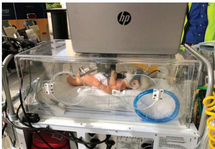
Figure 2. Simulated patient setting for recording sounds within the incubator during transport. Manikin in photo is wearing DREAMIES T-M device.
